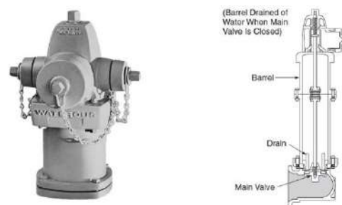
Figure 4-5: A Typical dry-barrel hydrant and its section.
