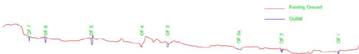
Figure 3-9: Existing Topography Section X-X showing invert level of PCR Outfalls.
