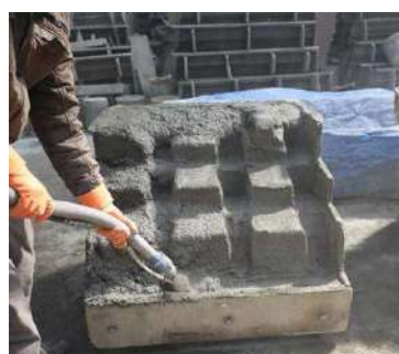
Figure 45 Surgical treatment of facade with the use of GRC cement.
